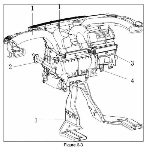
1. Air duct 2. Coolant pipeline 3. Blower 4. Heat exchanger
