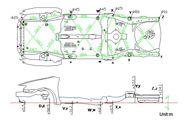
Front and rear shock dampers and sub-frame rear axle mounting holes coordinate:
