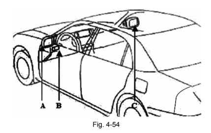
A: Left electric side mirror B: Electric side mirror switch C: Right electric side mirror
