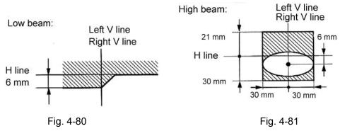
(4) Vertical focusing adjustment: Turn screw A for focusing adjustment using a screwdriver, to focus the light within designated range, when turning the screw A clockwise, the focusing light moves upward, contrarily, downward;
