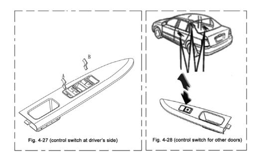
System operation: Operate the switch on door trim panel to make the window ascend or descend, as shown in Fig. 4-27 and Fig. 4-28. The driver can operate switches of all windows by operating the main switch on front door trim panel at driver's side; the safety switch of power window locates on front door trim panel at driver's side, the driver can inactivate the switches of all windows through key A. Only when the ignition switch locates at ON position, can the power window system work.
