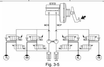
The pressure of wheel slave cylinder is maintained by the closed normally opened valve and normally closed valve, when proper pressure is applied to the salve cylinder through increase or decrease of pressure.
