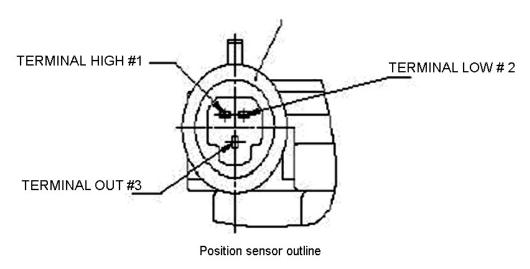
Pin: 1. Voltage input 2. Signal ground 3. Signal output
